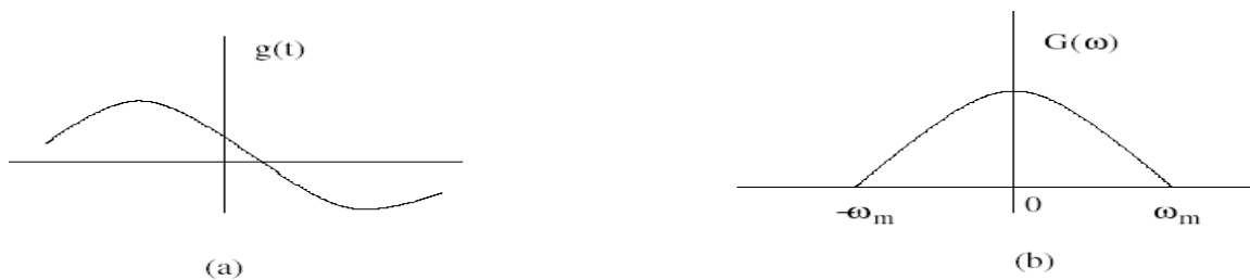
Figure 2: (a) Original signal g(t) (b) Spectrum G(\omega)
